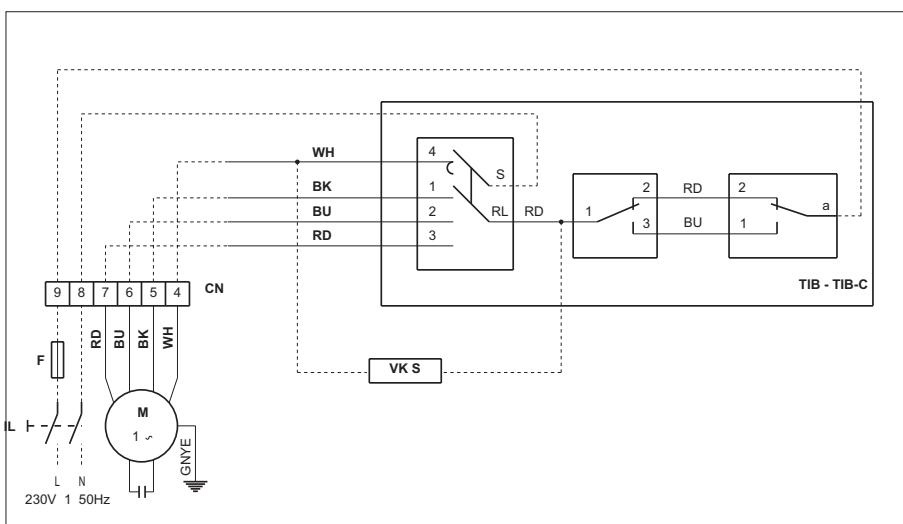
Each fan-coil requires a switch (IL) on the feeder line with a distance of at least 3 mm between the opening contacts, and a suitable safety fuse (F).
