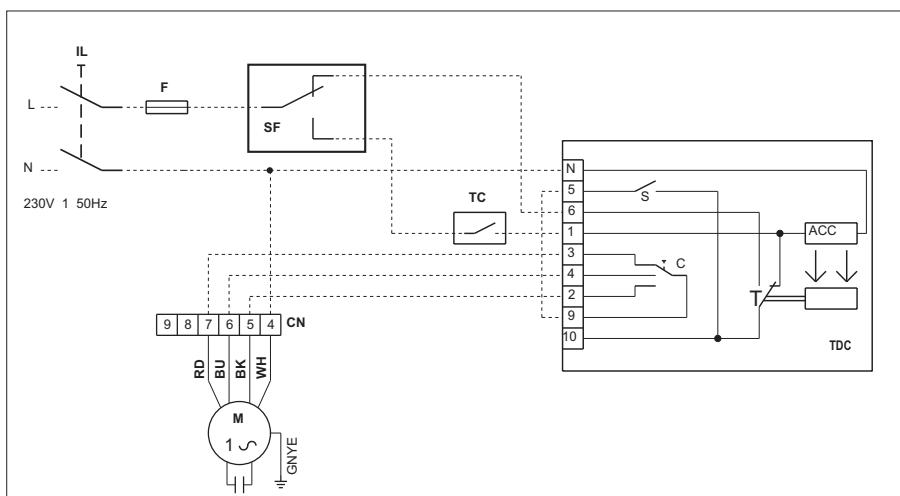
Each fan-coil requires a switch (IL) on the feeder line with a distance of at least 3 mm between the opening contacts, and a suitable safety fuse (F).
