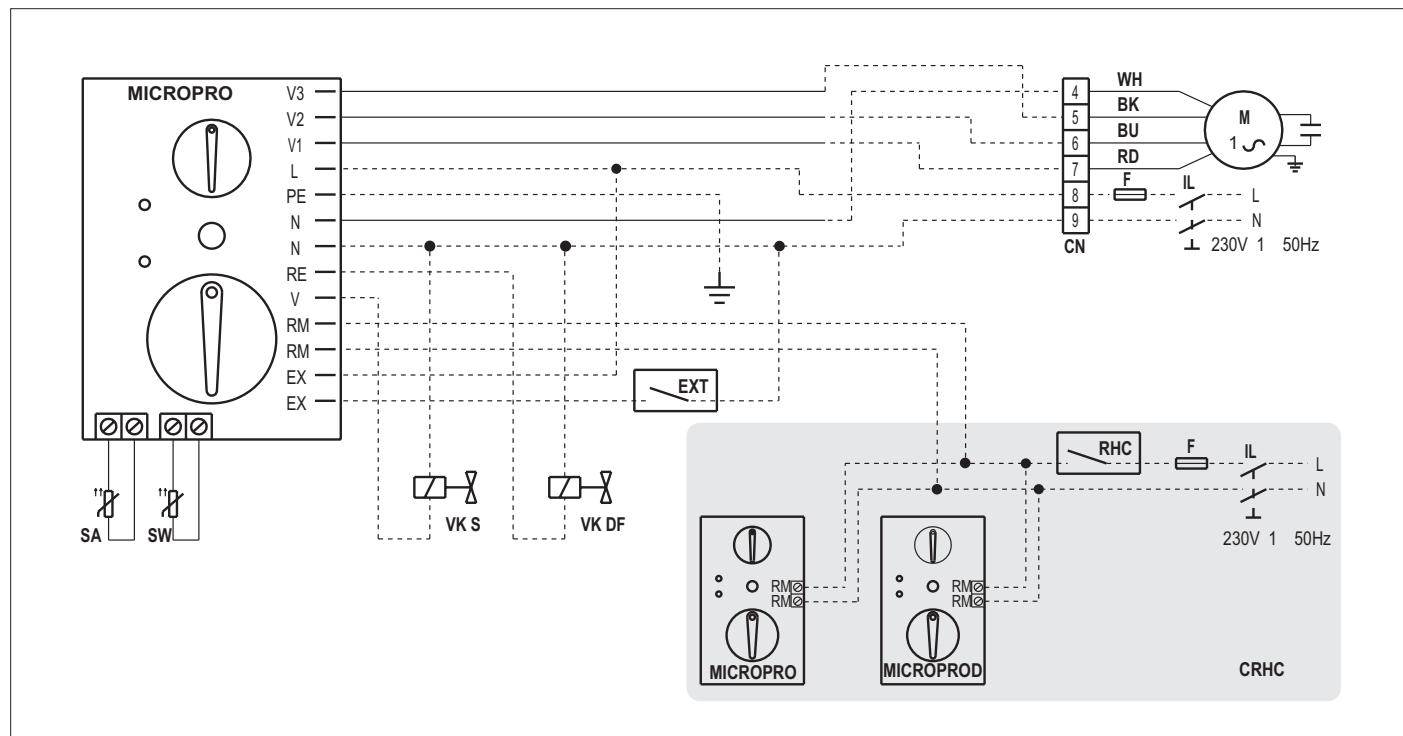
Each fan-coil requires a switch (IL) on the feeder line with a distance of at least 3 mm between the opening contacts, and a suitable safety fuse (F).
