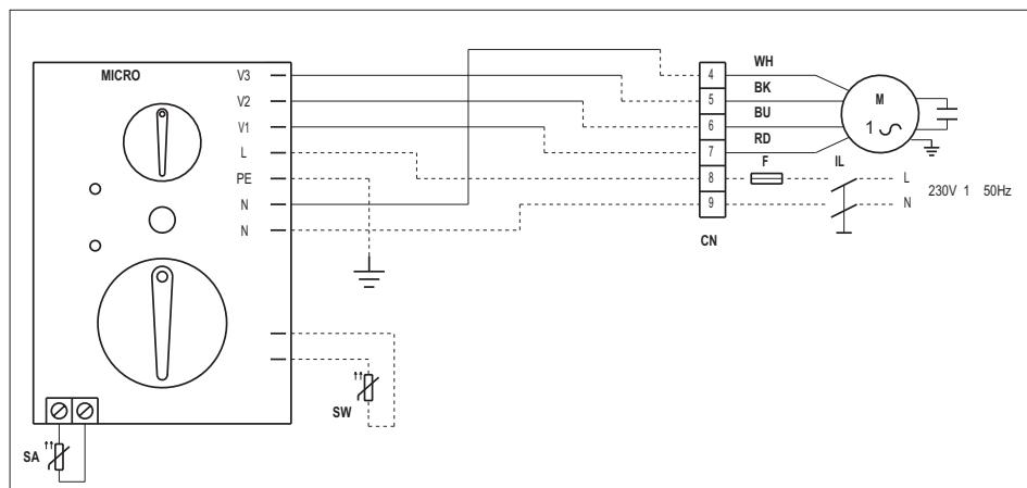
Each fan-coil requires a switch (IL) on the feeder line with a distance of at least 3 mm between the opening contacts, and a suitable safety fuse (F).
