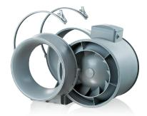
spigots by means of special clamps with latches. This makes the fan maintenance fast and easy. The fan maintenance does not require total disassembling. Just pull out the central block from the casing and perform required servicing. All the models may be equipped with a regulated timer with turn-off delay adjustable from 2 to 30 min.
